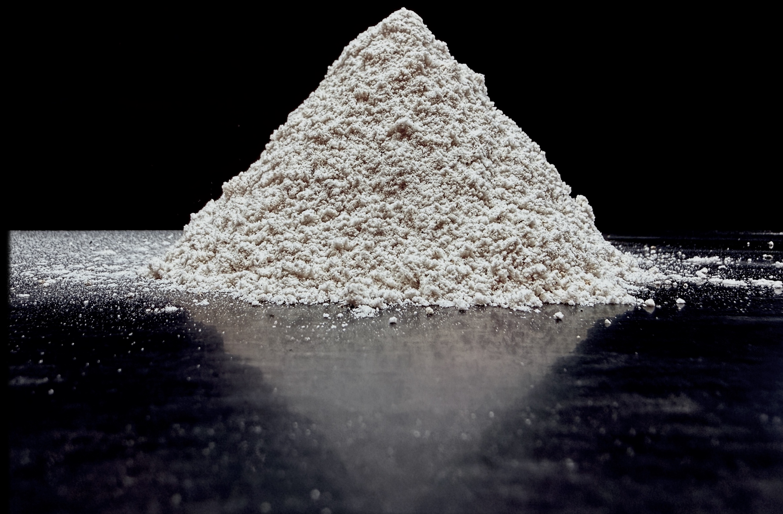
Figure 3. Lunar Low-Density (LLD-1) regolith simulant
